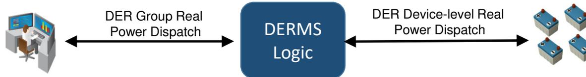
**“Strategy #1 - Uniform Distribution in Watts”:** Set/limit the active power level of each device in the DER group to the **same power level** in order to achieve the specified group power level.
