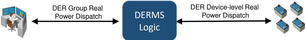
**“Strategy #1 - Uniform Distribution in Watts”:** Set/limit the active power level of each device in the DER group to the **same power level** in order to achieve the specified group power level.
