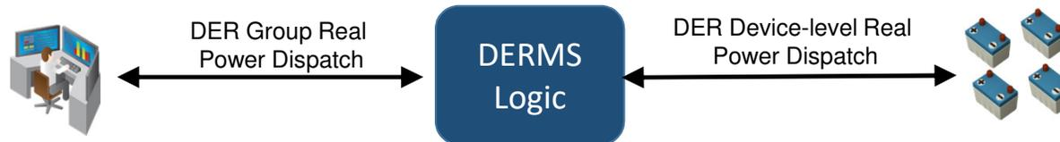
**“Strategy #2 - Uniform Distribution as a % of Nameplate Rating”:** Set/limit the active power of each device in the DER group to the **same % of nameplate rating** in order to achieve the specified group power level.
